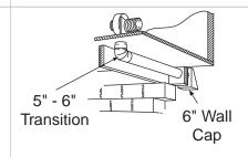
Down through the floor<sup>F</sup>, along the floor joists and through the foundation or an outside wall
